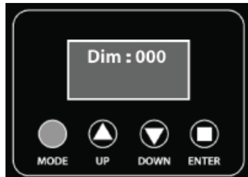
NO DMX CABLE CONNECTED
