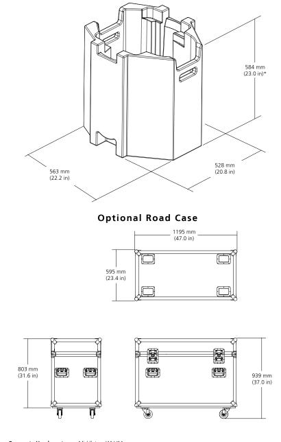
\*For Road Case consideration the metal base on the SolaFrame 1000 extends 13 mm (.5 in) higher than the highest part of the Molded Insert.
