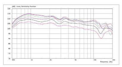
0/10/20/30/40/50 degree off-axis horizontal HF response (wide-axis).
