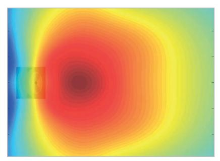
• LE200 SPL @ 4.5kHz over a 3 x 4m plane at head height Each contour represents 0.2dB change; yellow is -6dB
