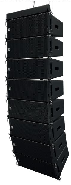
The cabinet has a PU paint finish with marine grade 316 stainless steel grille, flying hardware, fixings and pins. The exterior grille has an IP55 inner grille attachment and the HF and MF drivers feature Hydrophobic treatment and the LF and MF have a weatherised cone treatment. There is a weatherised cable gland with marine grade 316 gland and blanking plate and a 3m captive lead.
